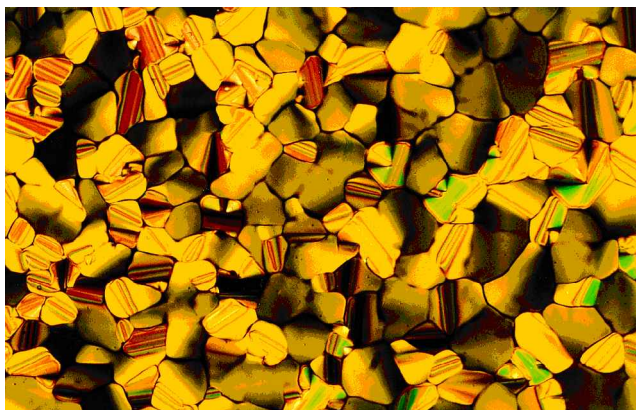
Figure 2. Texture observed by polarizing optical microscopy for the title compound at 160°C, obtained after cooling from the isotropic phase.
